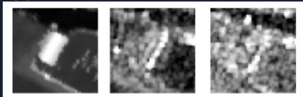
From left to right: Lidar image of an isolated building, double backscatter from TerraSAR-X in flooded conditions, and under normal conditions (Mason et al. 2014).
