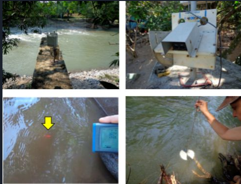
Clockwise from top left: TOF Lidar unit position along the Amacuzac River in Mexico; TrueSense S200 TOF Lidar, 64° incidence angle; Dispersion of laser light (indicated by the yellow arrow) in the water due to the Tyndall Effect; Researcher using a Secchi disk to assess turbidity (Tamari & Guerrero-Meza, 2016).
