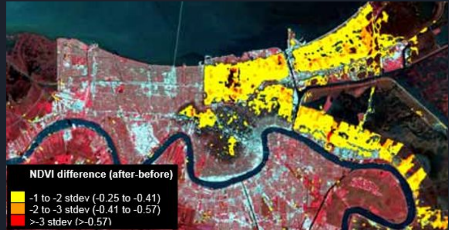
NDVI differenced images after masking of New Orleans. Higher standard deviations in NDVI indicate greater impact of flooding (Womble et al. 2006).
